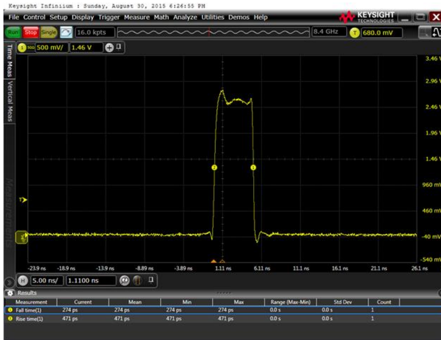
Figure 1: Pulses from the Comb are shaped and run into a driver circuit that creates a 470 ps rise and 270 ps fall time (typical).
